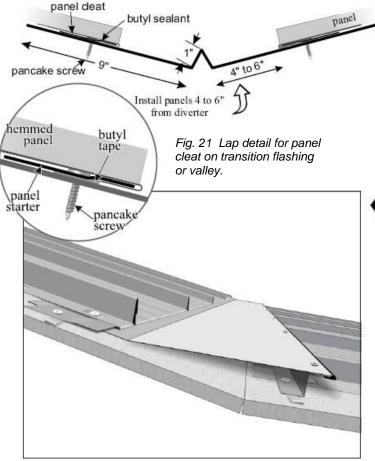
Fig. 22 Transition flashing combines the attachment techniques of valleys (top of page) with that used with ridge caps (p. 10). Notice the panel set-back that allows proper watershed from the upper panels onto the lower. The less the difference in pitch, as well as the flatter the roof, the greater the amount of set-back, and the more need for a longer "a" side on the transition flashing. The need is magnified even more for the higher-ribbed Gulf Seam panel.
