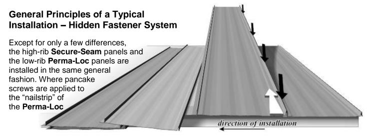
Fig. 8 Each Panel should be installed over the extended eave drip, pressed down and attached with the appropriate fasteners, and eave hems finished before installing the next panel.
