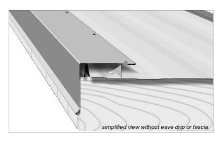
Fig. 17 Standard gable trim (EF-7) attaches to the z-flashing with rivets and to the fly rafter with either eave cleats (hidden fastener system) or exposed screws. The step rake option is shown below.
