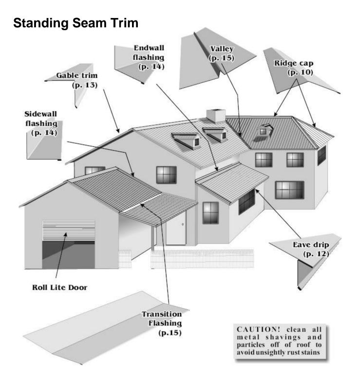
Fig. 6 Roofing trim and flashings are named by the location or function of that particular piece on the building
