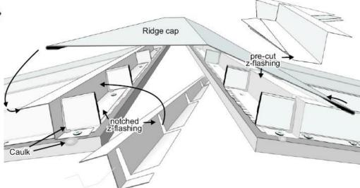
Fig. 11 To attach ridge caps, z-flashings are either notched (left) or cut into pieces (right) and mounted with screws at the upper ends of the panels. Caulk is applied on the bottom side and around the panel ribs to seal the ridge against rain. The mounted ridge cap is attached to the z-flashing with rivets.
