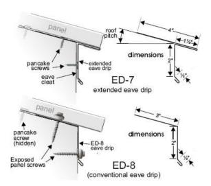
too steep). If more than one pitch is involved, specify the number of each pitch (eave drip comes in 10-foot lengths). Order 90 degree eave drip for square-cut eaves.
