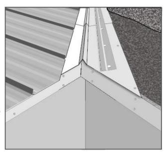
Fig. 20 Diagonally-cut panels are hemmed and attached to panel starter that is mounted on the surface of the valley.
