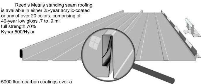
urethane primer of .2 to .3 mil on the finish side, with primer and washcoat on the reverse side. Metallic coatings are also available and carry the same 40-year warranty. We manufacture both stock and custom trims and flashings, and provide
