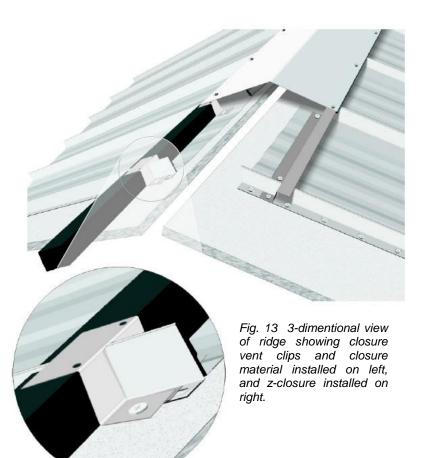
When attic ventilation is desired, vent clips can be used in the place of z-flashing. Vent clips straddle each rib, and support the ridge cap in much the same manner as the z-flashing. Closure material is inserted between the ribs and sandwiched between the panels and the ridge caps. The decking must, of course, be cut at the ridge to let out hot air.
