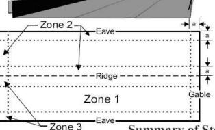
Fig. 23 Note: Dimension **a** is defined as 10% of the minimum width of the building, or 40% of the mean height of the roof, whichever is smaller; however, **a** cannot be less than either 4% of the minimum width of the building, or 3 feet.
